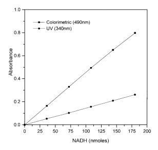
**FIG. 1.** Comparison of the standard curve of NADH measured by tetrazolium reduction with that of UV absorbance. Graded concentrations of NADH were reacted with iodonitrotetrazolium in the presence of PMS in Tris buffer (0.1 M, pH 7.4). The color was measured at 490 nm and plotted with the absorbance of NADH at 340 nm. Each point is the mean of triplicate values.
